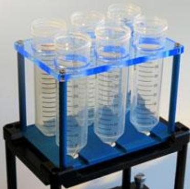
The labware import file contains two definitions, seen at right. In both cases the tube holder is defined as a reservoir with six sections. The circular cross section of the tubes was translated into rectangular sections with the same area. This leaves volume calculations and liquid level tracking intact.<sup>1</sup>
